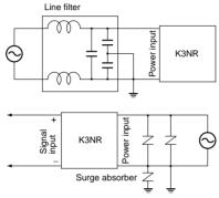
In order to prevent inductive noise, wire the lines connected to the terminal block separately from power lines carrying high voltages or large currents. Also, do not wire in parallel to, or in the same cable as power lines. There are other methods that are effective for reducing noise, such as running wires along ducts and using shield lines.
